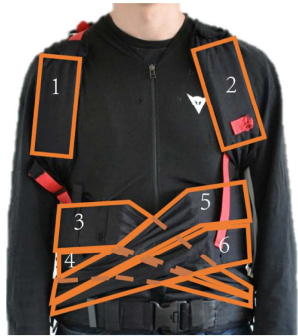
a.) The soft robotic vest. Actuators marked 1-6
