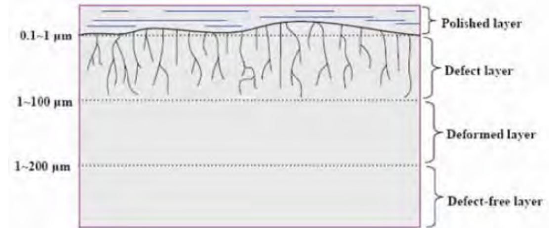
Residual cracks in optical materials
